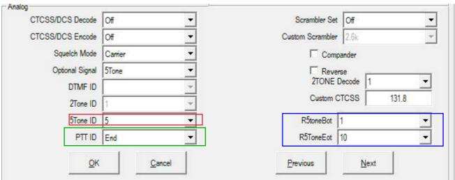
In PTT ID it is possible to decide whether to send a sequence when pressing the PTT, when releasing or both
