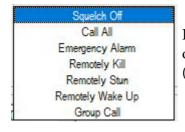
In addition to these functions it is possible to associate a sequence to remotely turn off the radio (Remotely Kill), to turn it back on (Remotely Wake Up) or block it (Remotely Stun) but be careful when using these commands
